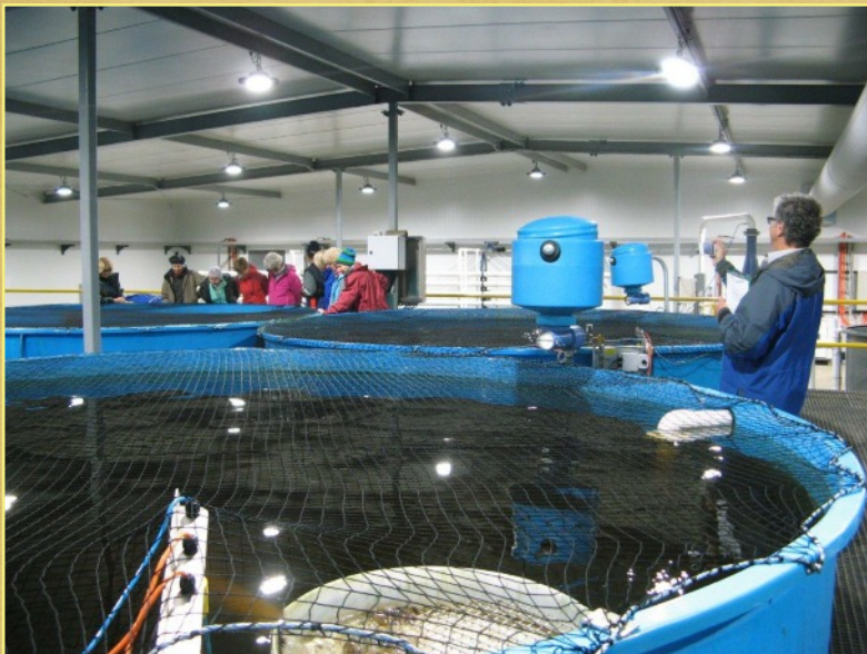
Tanks like this hold the young fish as they develop. The amount of feed required has been calculated for the different stages of development and is fed automatically at optimum intervals. The pellets are 50% protein. The waste [feed and excretion] is sucked off the bottom, and transferred to a tank where it is fed to bacteria and ultimately returned to a pH of 7.
