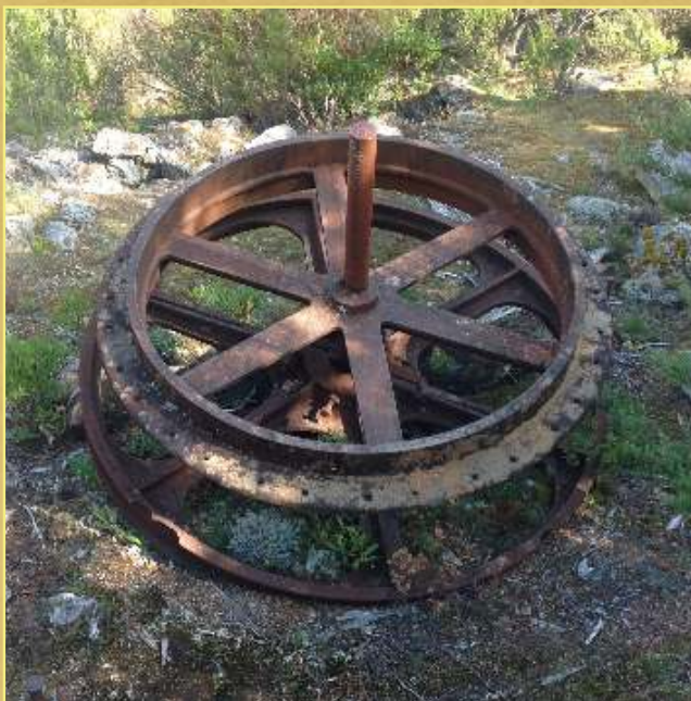
The 'bull wheel' - part of the haulage line used to move tin to the Anchor Mine for processing (CFE)
